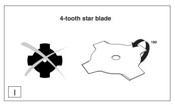
Note: The cutting tools below should be sharpened <u>only</u> at a <u>qualified workshop!</u> Manual resharpening will result in an imbalance of the cutting tool, causing vibrations and engine damage.
